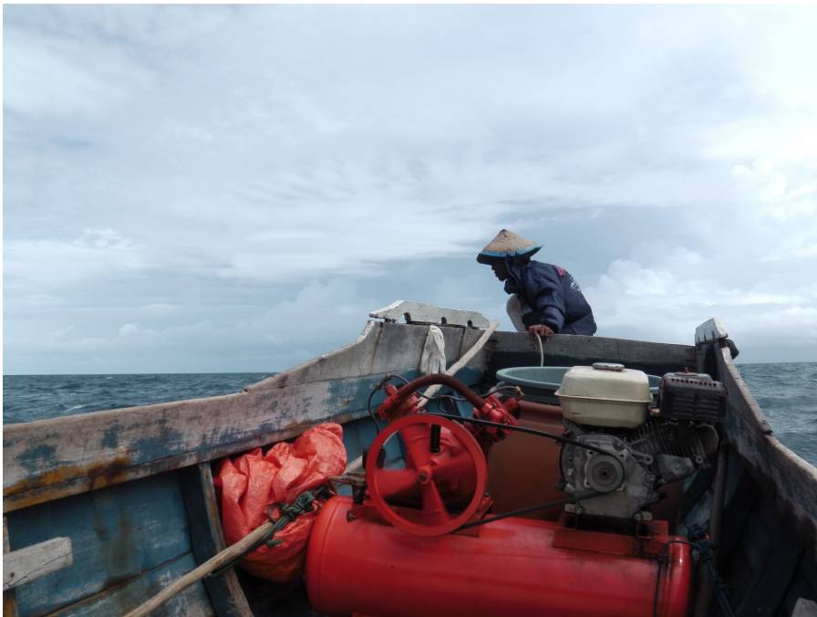
Figure 1. A fisher keeps the oxygen tube under a little strain, safeguarding the air flow between the air compressor and the diver below the water surface. Photo by the author.
